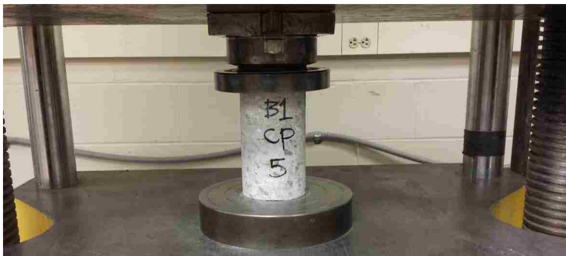
Figure 5.19 Compressive strength test setup of cores.
