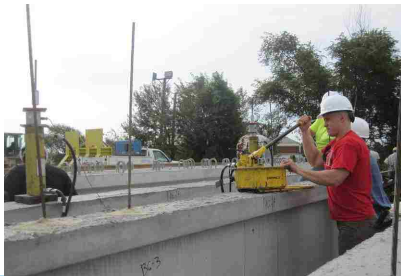
Figure 5.25 Strands being tested using pull-out test.
